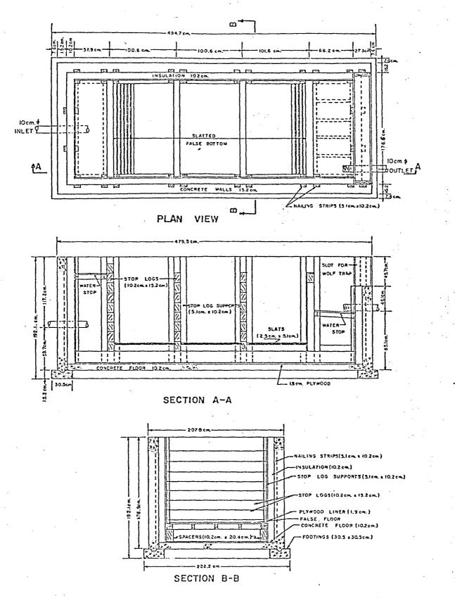
Fig. 2. Diagram of the "Exploits River Box".
